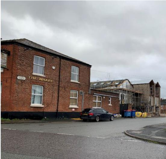
This building is too low to provide the necessary coverage to the target coverage area. It also has a hipped roof which is unsuitable for a telecommunications installation. There is insufficient space in the yard area to accommodate a radio base station at this location. A site at this location has therefore been discounted.
